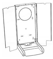
**3.** Mount the wall bracket securely in the desired position. ONLY USE FIXING MATERIALS, WHICH CANNOT MELT.
