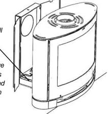
**6**. Secure the stove by mounting one screw on the top and one in the bottom. Note: You will find the screw for the bottom of the stove in the ashpan.
