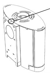
**1.** Dismount the security screw and pull the wall bracket from the stove.
